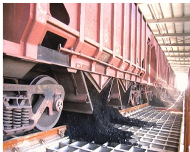
FIG 4 TRACK HOPPER UNLOADING SYSTEM
