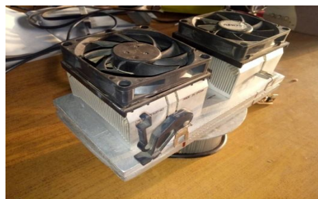
Fig: 6 Experimental Setup using a thermoelectric modules model TEPI-1264-1.5 Between a Controlled hotplate and a cooling fan
