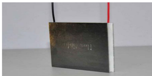
Figure 1: (a) Thermoelectric device(model TEP1-1264-1.5)
