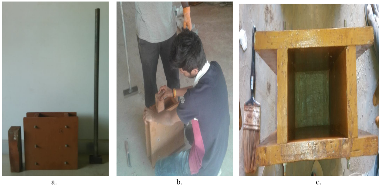
Figure 5 a. A rectangular rammer, wooden mould and wooden logs. b. To ensure the thickness of each layer by using the wooden log. c. Bonding between the layers cement paste is used.
