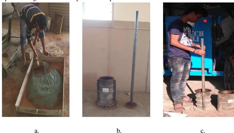
Figure 5 a. soil and cement were mixed thoroughly in dry state, b. A circular rammer, cast iron metal mould, c. Compacting soil mixture
