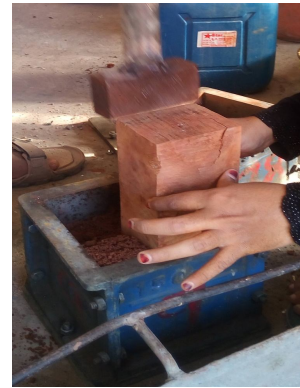
Figure 9 Compacting wet soil with rammer
