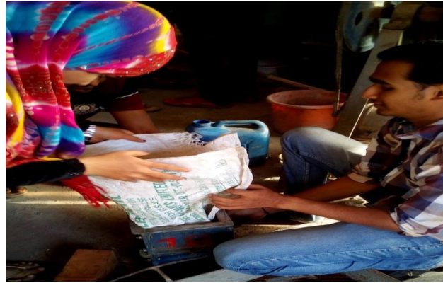
Figure 7 Pouring wet soil per layer
