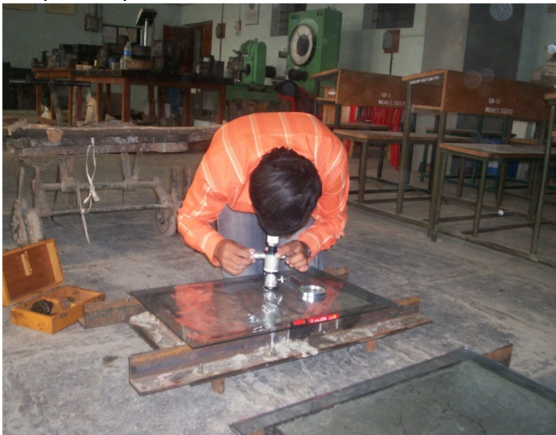
Fig.1. Shows the measurement of crack width by using Hand Microscope
